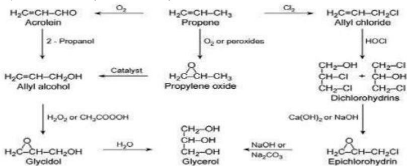
\* Epichlorohydrin process is most important, as it involves the chlorination of propene to give allyl chloride, which is oxidized with hypochloride to dichlorohydrins, which further reacts with strong base to give epichlorohydrine. Epichlorohydrine is a chlorohydrine of propene to give GLYCEROL
